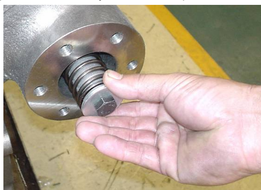
Unloader (device spring and push rod)
