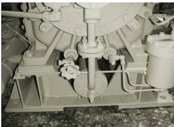
Bottom-type oil tank (connected by flanges to the crank case)
