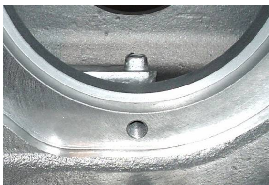
Position of the protrusion of the unloader push rod (when it is at the bottom)
