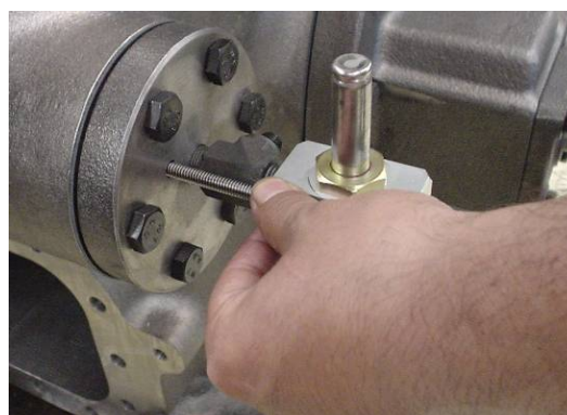
Position adjustment of the unloader push rod
