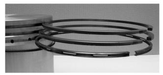
Fit the piston rings and oil scraper in the orientation as Fig.81: shown
