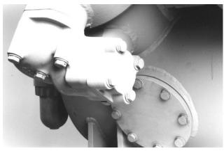
Fig.9: Back pressure dependent relief valve
