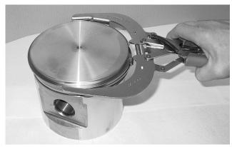
Fig.76: Remove the piston rings and the oil scraper ring (tool not in tool set)
