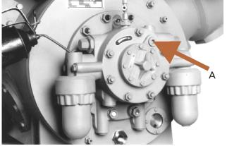
Fig.166: Oil filters and location oil charge valve (A); not shown!
