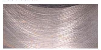
Fig.139: New honing profile and crosshatching with the right angle
