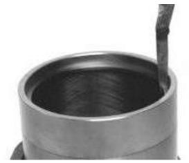
Fig.78: Check the gap in each piston ring by placing it in an unworn part of the cylinder liner. These unworn parts can be found at about 10 mm from the bottom of the cylinder liner. The maximum gap as given ()
