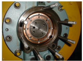
Fig.128: Standard thrust bearing; refer also Figure 38, Page 25
