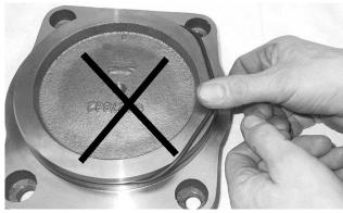
Fig.179: WRONG WAY OF MOUNTING
