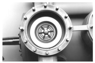
Fig.153: Top view of discharge valve assy
