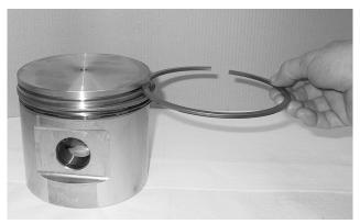
Fig.77: Replace the NEW piston rings; Roll each piston ring and oil scraper ring in the corresponding groove around the piston to trace parts that have become wedged.
