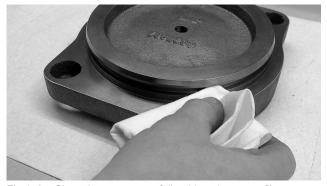
Fig.176: Clean the groove carefully with a clean, non fibrous cloth
